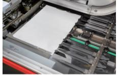
After transport to the nipping section, the cover is registered precisely with the fore-edge guide and tail-edge positioning guides.
