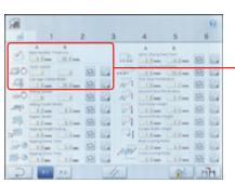
Customized templates can be created according to desired book quality, paper type and other factors. These customized templates can be created by a key operator or manager who controls the quality. Once a template is created, the operator just selects the desired template to setup the system. This enables any operator to produce consistent quality books with improved production efficiency and greater quality control.
