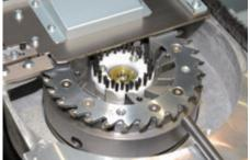
Powerful servo motor driven milling and notching mechanism mills the spine of the book block or signatures for optimum glue penetration and adhesion. Milling rotation speed can be adjusted automatically according to book thickness and custom templates. Milling depth can be adjusted from 0 to 4 mm or 0" to 0.157".
