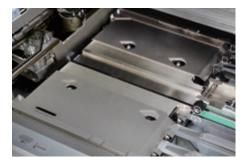
A strong rigid nipping mechanism and positive jogging guarantees precise alignment of the cover to the book block and square spines. Nipping width, height, operating time and delay time are adjusted automatically according to book thickness.
