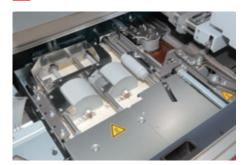
Dual application rollers and side gluing rollers ensure superior glue application to the spine and excellent adhesion of the cover for consistent quality binding. Glue roller height, wiper opening and cut-off timing, scraper roller height, and side glue roller width are automated.
